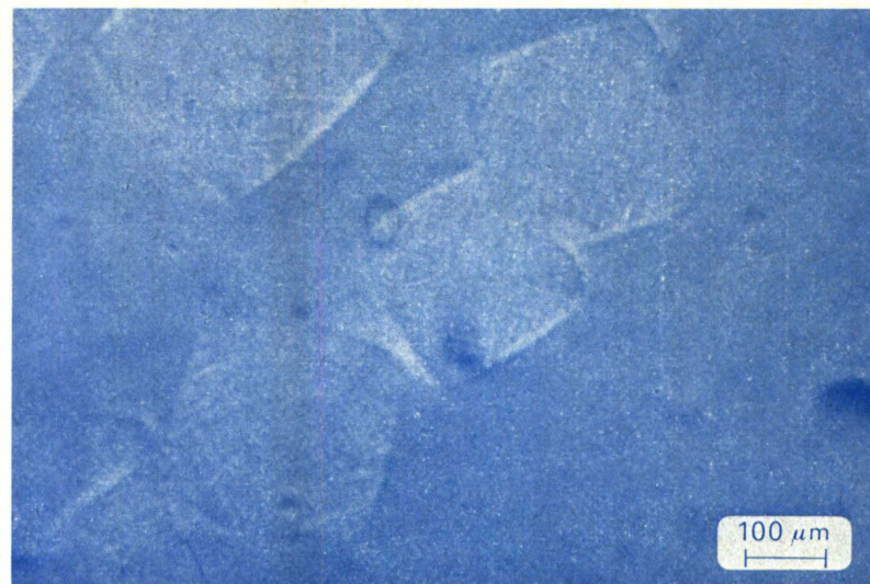
Fig. 2. Liquid single crystals of cholesteryl decanoate (90.45 °C) showing the cross-hatching of BP I. Sample thickness 12 μm (in transmission).
